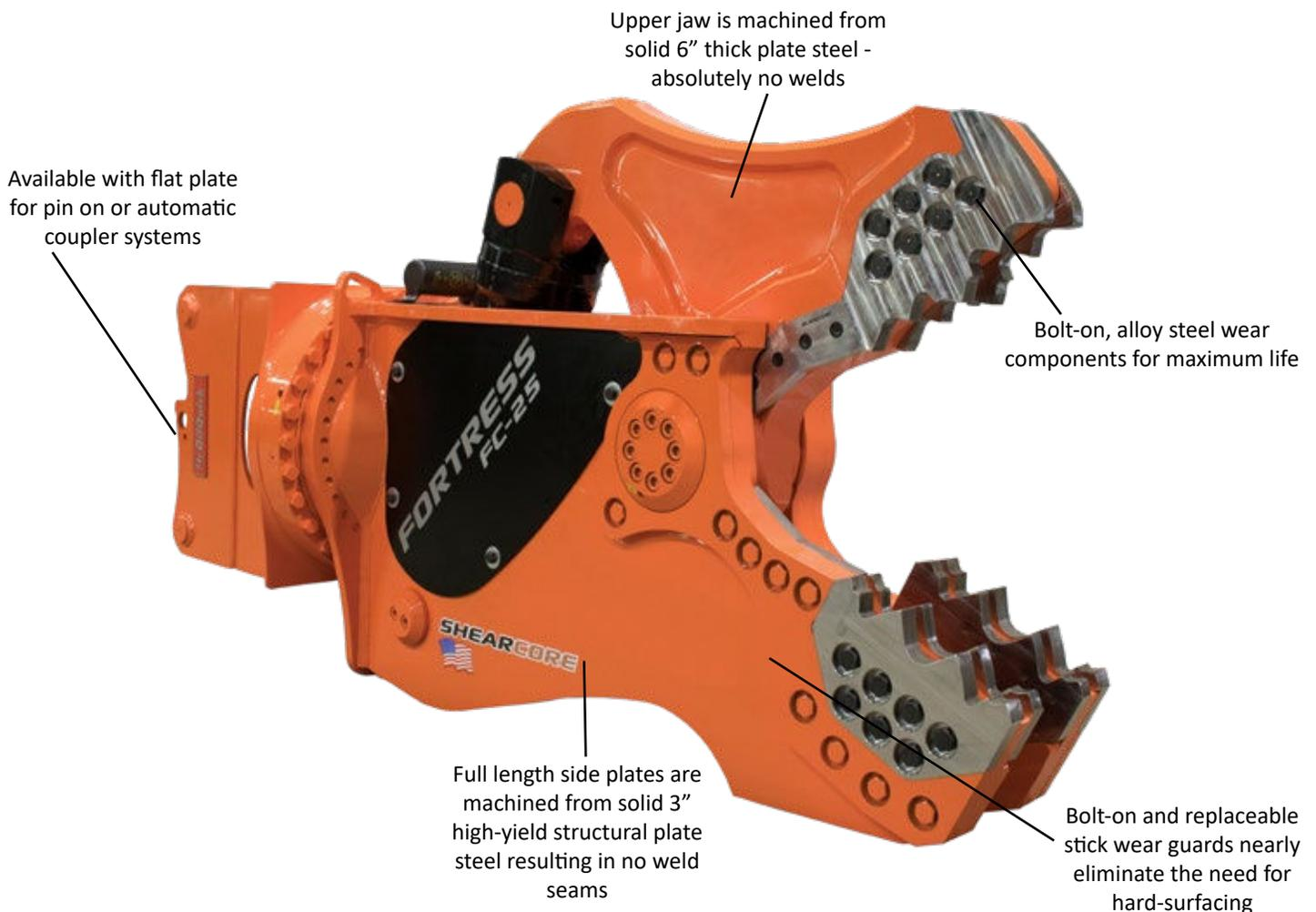
**Why call it a Demolition Shear?** The Fortress FC is a new class of tool with unique construction and capabilities. It utilizes a solid upper with no welds and press-fit pivot group (like our shears) allowing for tolerances tight enough to shear rebar all the way out to the tip.
